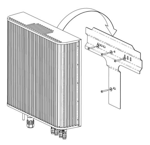
When correctly in place and seated on the wall bracket, the bottom end of the Inverter should swing back over the locking tab.
