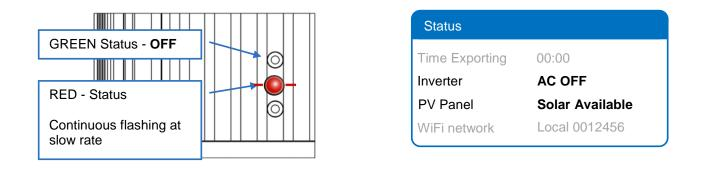
AC mains OFF Check AC Isolator switch adjacent to the Inverter and/or the circuit breaker in the Switchboard.
